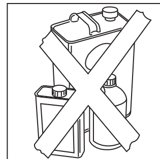
Fig. 3 - NO combustible materials near furnace
