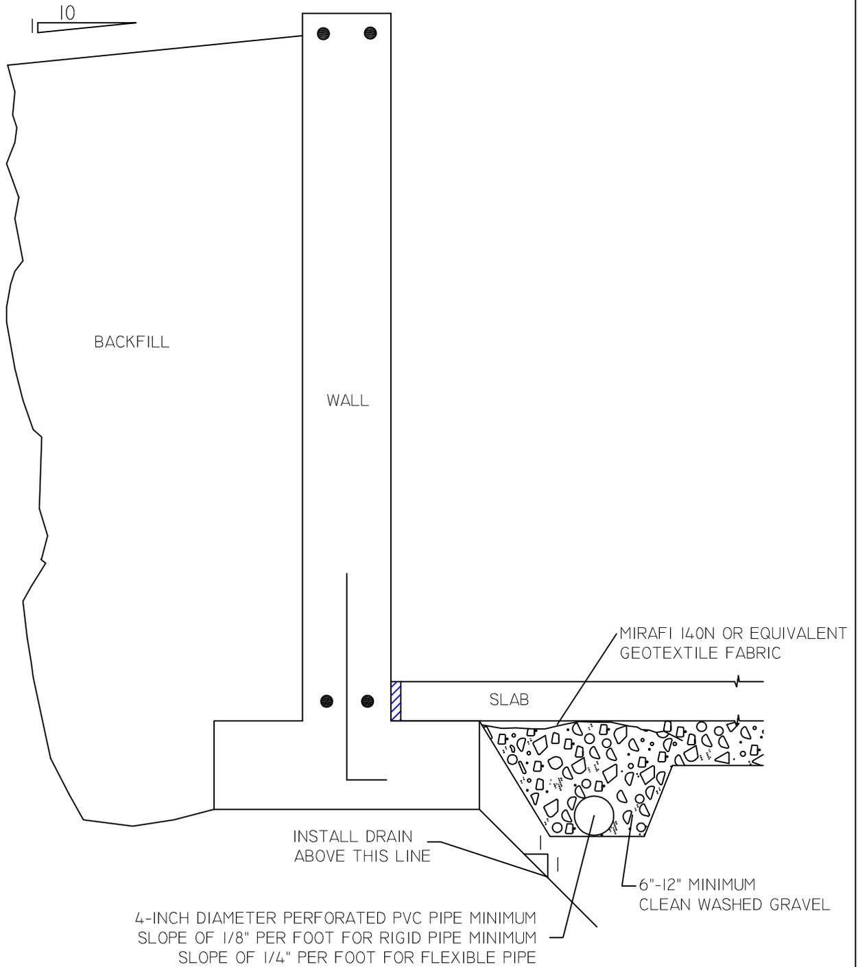
4-INCH DIAMETER PERFORATED PVC PIPE MINIMUM SLOPE OF 1/8" PER FOOT FOR RIGID PIPE MINIMUM SLOPE OF 1/4" PER FOOT FOR FLEXIBLE PIPE
